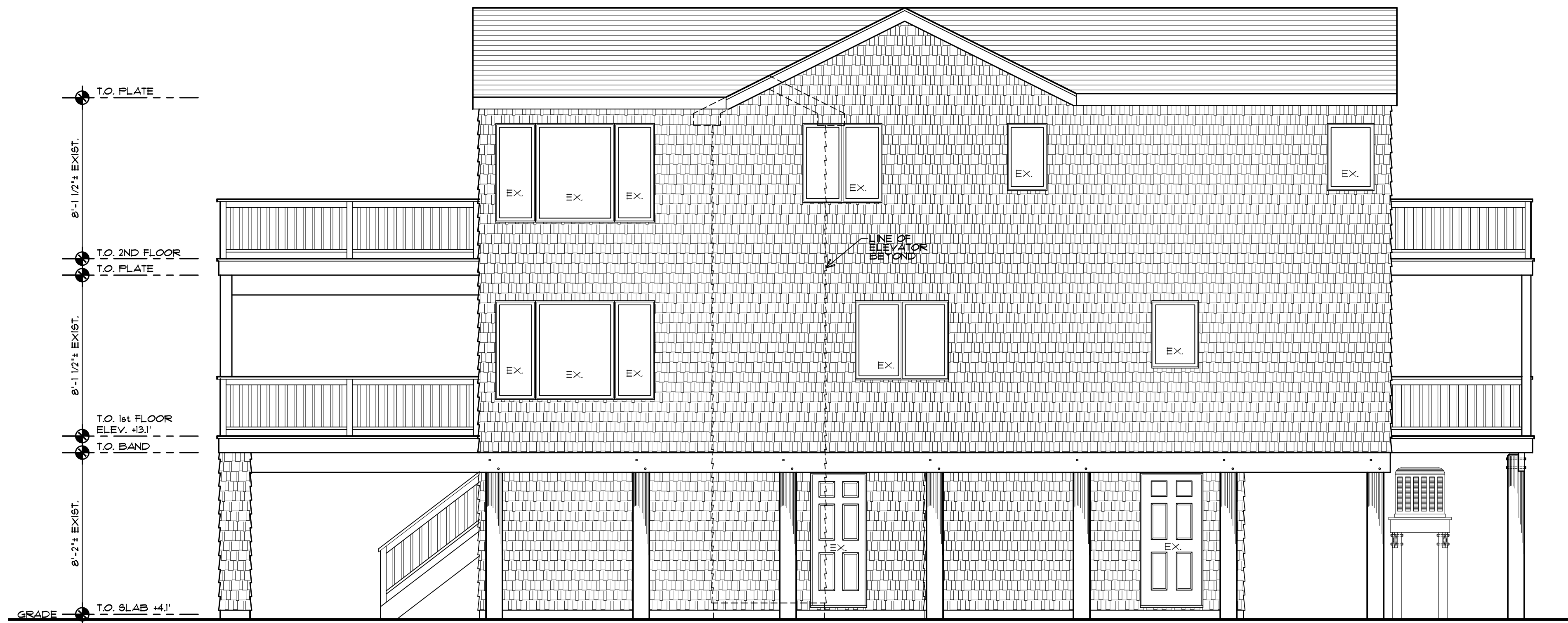
RIGHT ELEVATION (WEST SIDE) 1/4" = 1'-0"
